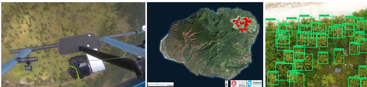
Fig. 1. (Left) Prototype Helicopter-mounted camera mapping system. (Center) Mapping results from helicopter survey of >9,000 hectares on Kaua'i island. (Right) Plant detection results from convolutional neural network algorithm applied to high-resolution (<5 cm) sUAS imagery.
